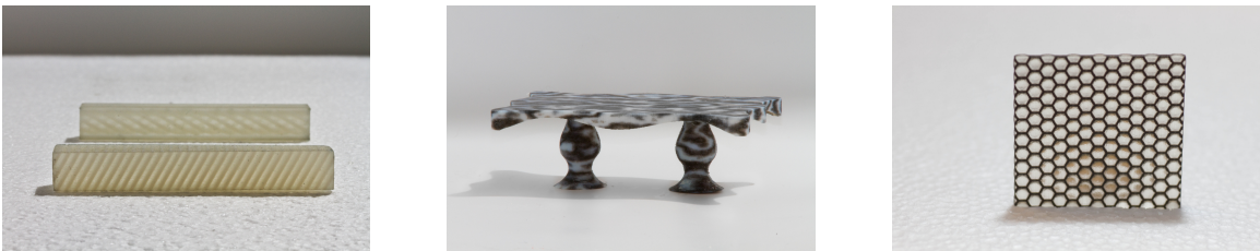
Figure 7-5: Left : procedurally-defined materials with anisotropic mechanical properties. Center : Marble-like material generated using Perlin noise. Right : Procedurally-defined and fully parameterized aspherical microlens array with baffles.
