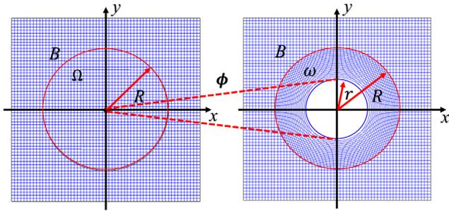
FIG. 1. Schematic representation of the transformation method:  $\Omega$  is a fictitious reference medium and  $\omega$  is the physical medium; transformation  $\phi$  maps a point of the reference into a circular area of radius  $r$  hosting the cloaked object while leaving unchanged the background beyond a distance  $R$  from the center; the remaining annulus of thickness  $R - r$  hosts the cloak.
