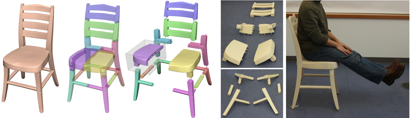
Figure 1: Chopper partitions a given 3D model into parts that are small enough to be 3D-printed and assembled into the original model. Left to right: the input chair model, Chopper’s partition (with a printing volume shown as a reference), printed parts, and assembled chair.
