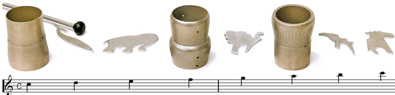
Figure 1: Customized instrument. A set of optimized 2D water jet cut animals and 3D printed cups form a musical scale. Provided with a user-supplied 3D shape and target sound characteristics of the desired frequencies and their amplitudes, our method optimizes the geometry of the object to realize the desired sound (see video).
