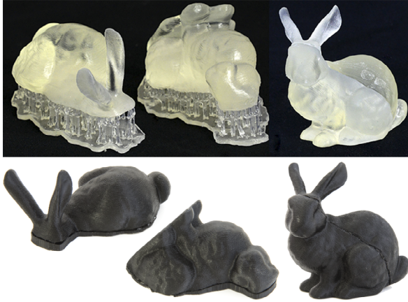
Figure 12: The bunny has been segmented into two parts with limited overhang angle and printed with the Form 1 STL printer (top) and the Ultimaker 2 (bottom). No support is needed for the surface.
