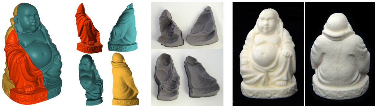
Figure 1: To fabricate a mesh, possibly acquired by laser scanning, in a molding process, we automatically decompose and deform the shape (center left). A reusable multi-piece mold for the object can be produced by CNC milling (center right). Physical copies can be fabricated by mold casting in different materials like resin or plaster (right).
