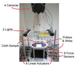
Figure 2: Acquisition setup for the measurement system.
